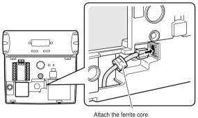
Attach the ferrite core supplied to the LAN cable.
